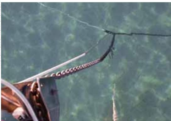
*A Bahamian moor: two anchors laid off the bow, on two cables joined by a snatch block. It's secure, but hard to lay and recover*
